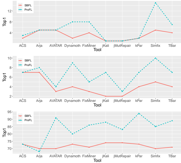
Figure 9: Unified debugging on buggy versions with (1) correct, (2) incorrect but plausible, and (3) implausible patches
